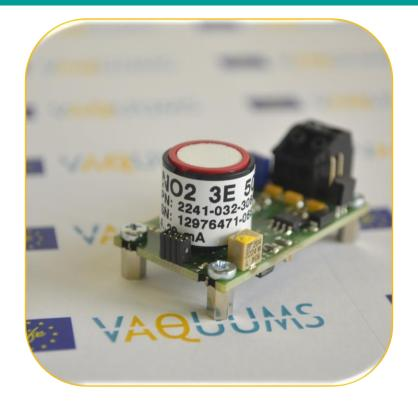
The Citytech NO2 3E50 is an electrochemical nitrogen dioxide sensor. According to the manufacturer it can measure concentrations between 0 and 50 ppm. It is mostly used for industrial applications.
